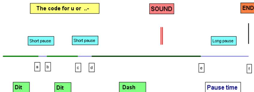
Figure 2. Drawing of a time line of the code for 'u' with a single switch. Moments **a** to **f** are marked, and the next code starts at **g**, not displayed because with novices it is far to the right of this page. Proportionally, all pauses are somewhat longer than is shown.
