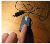
Picture 1. Switches discern subtle body movements and may be connected to a special mouse.
