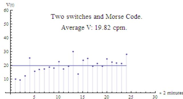
Figure 6. Learning curve with a healthy test subject, two switches, a copy task and *one* hour of previous training. Pause time was 280 milliseconds, somewhat higher than strictly necessary, to reduce the number of errors. All errors had to be corrected and pause time was *not* varied.
