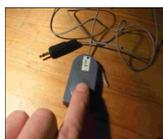
Picture 1. Switches discern subtle body movements and may be connected to a mouse or to specialized input gear.
