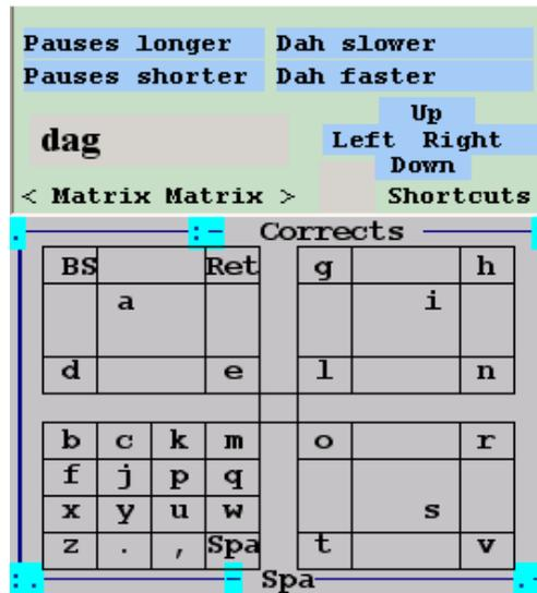
Figure 12. Redesign for a single switch with a frequency-optimised matrix.
