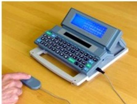
Photo 3. A model with a single switch and a scan unit that supports row column scanning and also stepped scanning with integrated word prediction.
