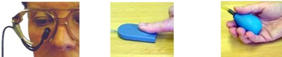
Photo 1. Several switches to record blinking (with an infrared light), clicking and pressing.
