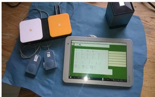
Picture 2. Left and Right switches are connected to blue tooth switches, that sit in Froggy's belly with the blue tooth speaker.
